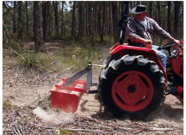
Bulldozing - The back-blade acts as a dozer when the tractor is reversed, which is particularly useful for pushing up rows.
