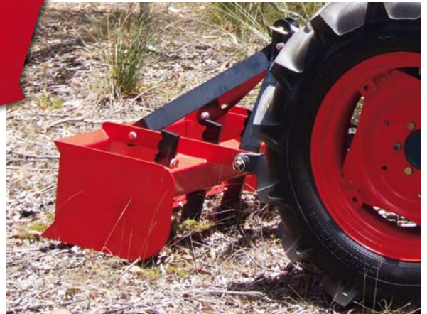
Scarifying / Ripping - The heavy box frame enables the tines to effectively "bite" into the ground, minimising bouncing on hard ground.
